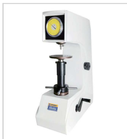
200HR-150 洛氏硬度计 Rockwell Hardness Tester
